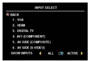
VGA — Select when you have your computer connected to the VGA connector. See "Bottom View" on page 7 for the location of the VGA connector.
